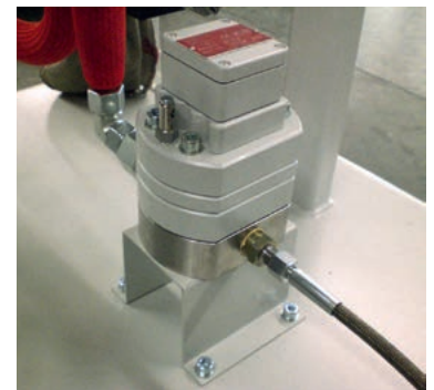
▲ volume counter for metering control and automatic readjustment
