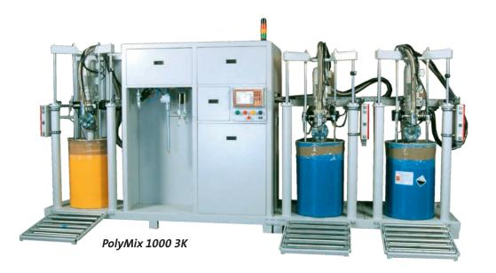
Electrically actuated metering unit for the processing of high-viscosity EP and PUR bonding paste
