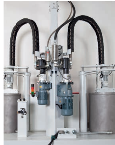
▲ back view with supply couplings, gear metering pumps, flow meters and pressure regulators for floating follower plates.
