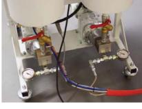
is fitted with pressure manometers and non return valves, providing the operator with more application information.
