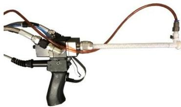
The *PGM system* uses disposable static mixers and a plastic moulded air cap to atomise the material and transfer the product from the static mixer into the mould or onto the parts. With a pot-life of less than 45 seconds the product can be demoulded or sent to the next stage of production.
