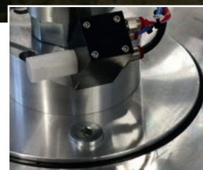
▲ integrated roll-in-device with automatic barrel bottom support
