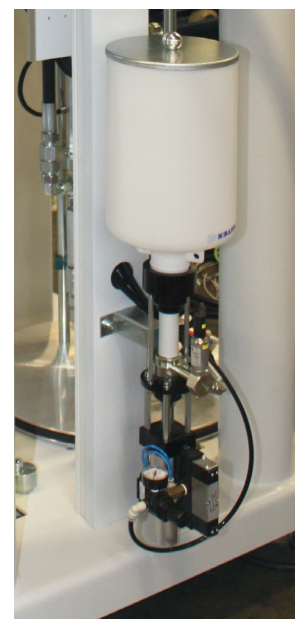
10 l feeding pump for colour with empty control indicator
