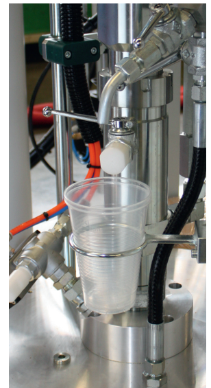
Cupholder for air venting
