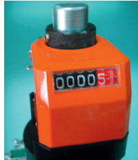
colour metering with metering valve and position indicator
